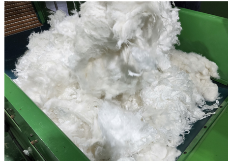
Fig. 5. Hemp stem shell 20% Riocell 80% mix.
